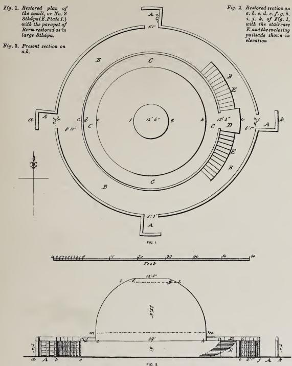
N.B.—The dotted line l.l. shows the top diameter, of 19', as measured by Capt. Fell, in 1819. m.m., 3' 6'' above the basement, is the line whence the curve springs.
